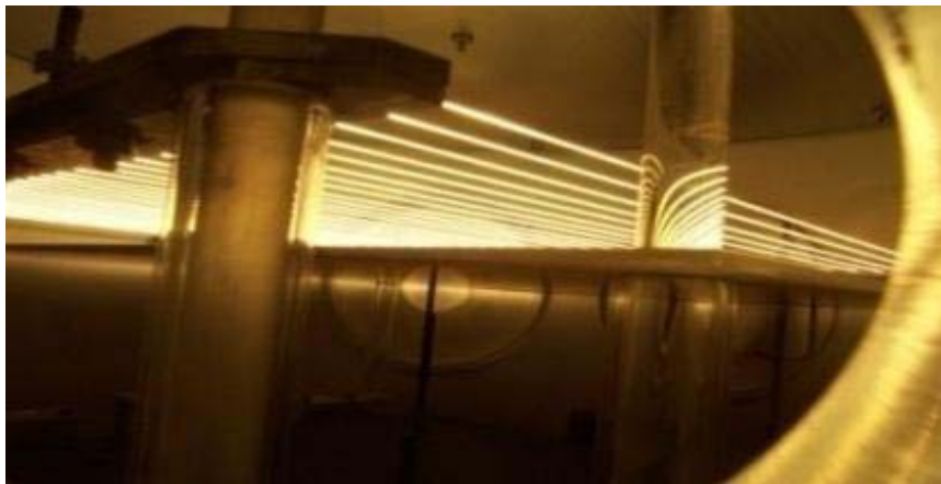
Figure 3.2.1. A hot filament CVD reactor at advanced diamond technologies (ADT).
