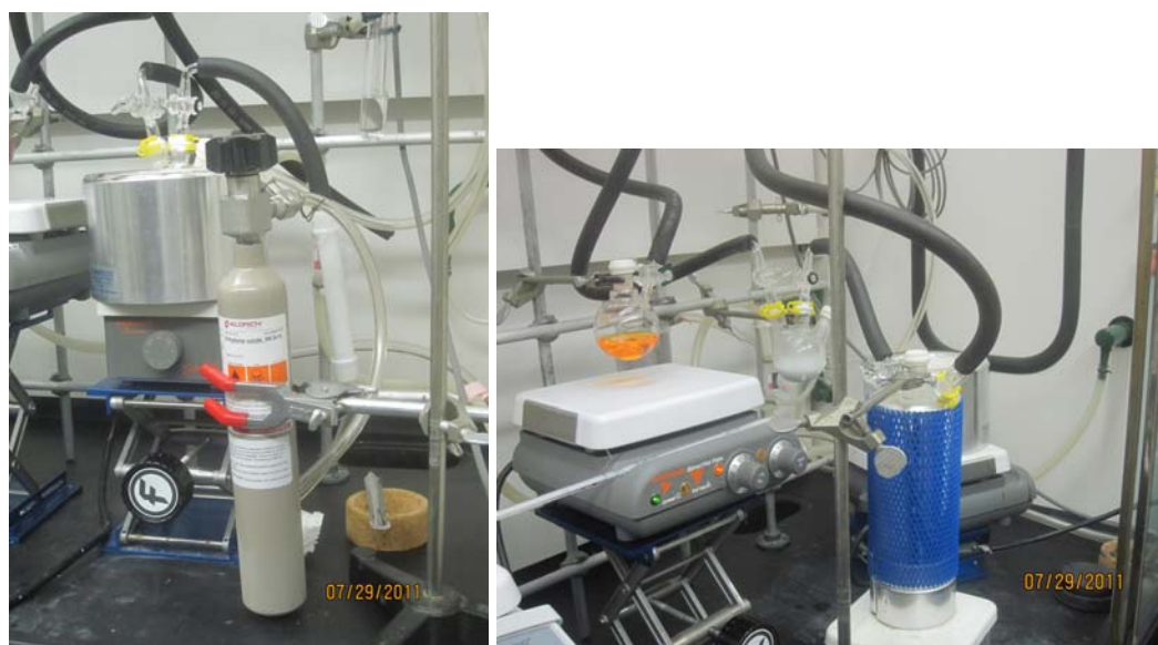
Figure 16. Pictures to show the experimental set-ups to collect ethylene oxide (left) and the cryo-distill the collected ethylene oxide into a graduated Schlenk tube (right).
