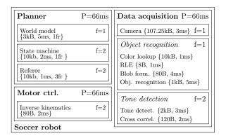
Figure 1. Software modules of a soccer robot.
