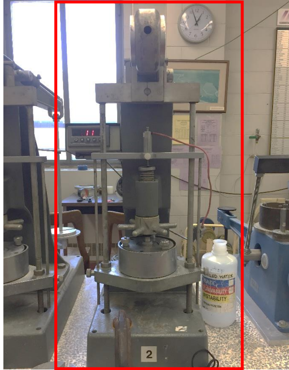
Figure 3. 1 The consolidation test unit
