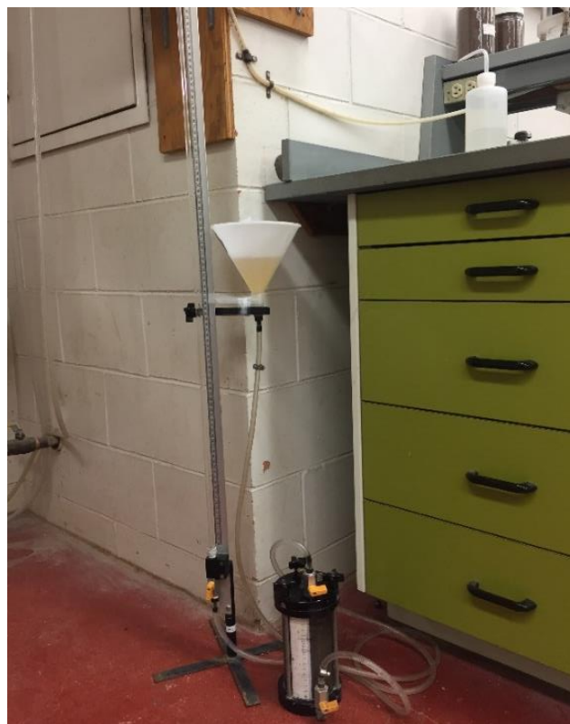
Figure 3. 4 Falling head test apparatus
