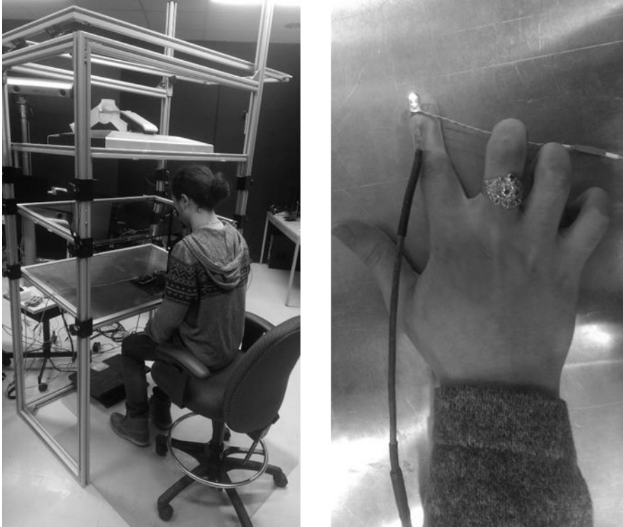
Figure 2. Aiming apparatus (left panel) and close-up view of LED and IRED placement on the reaching limb. The LED was necessary because the combination of the one-way mirror and extinction of the lights in the experimental suite prevented direct vision of the reaching limb.
