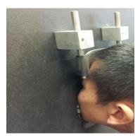
• Adjust forehead rest by unlocking screws (move rods up/down and lock screws).
