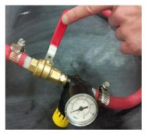
• Attach hose coupling to the 40 psi air line at the workbench
