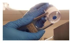
Check each tube is hanging over a white hook and string at the box roof. This step ensures the cassette will be at the correct distance from the cough inlet and on the box centreline.
