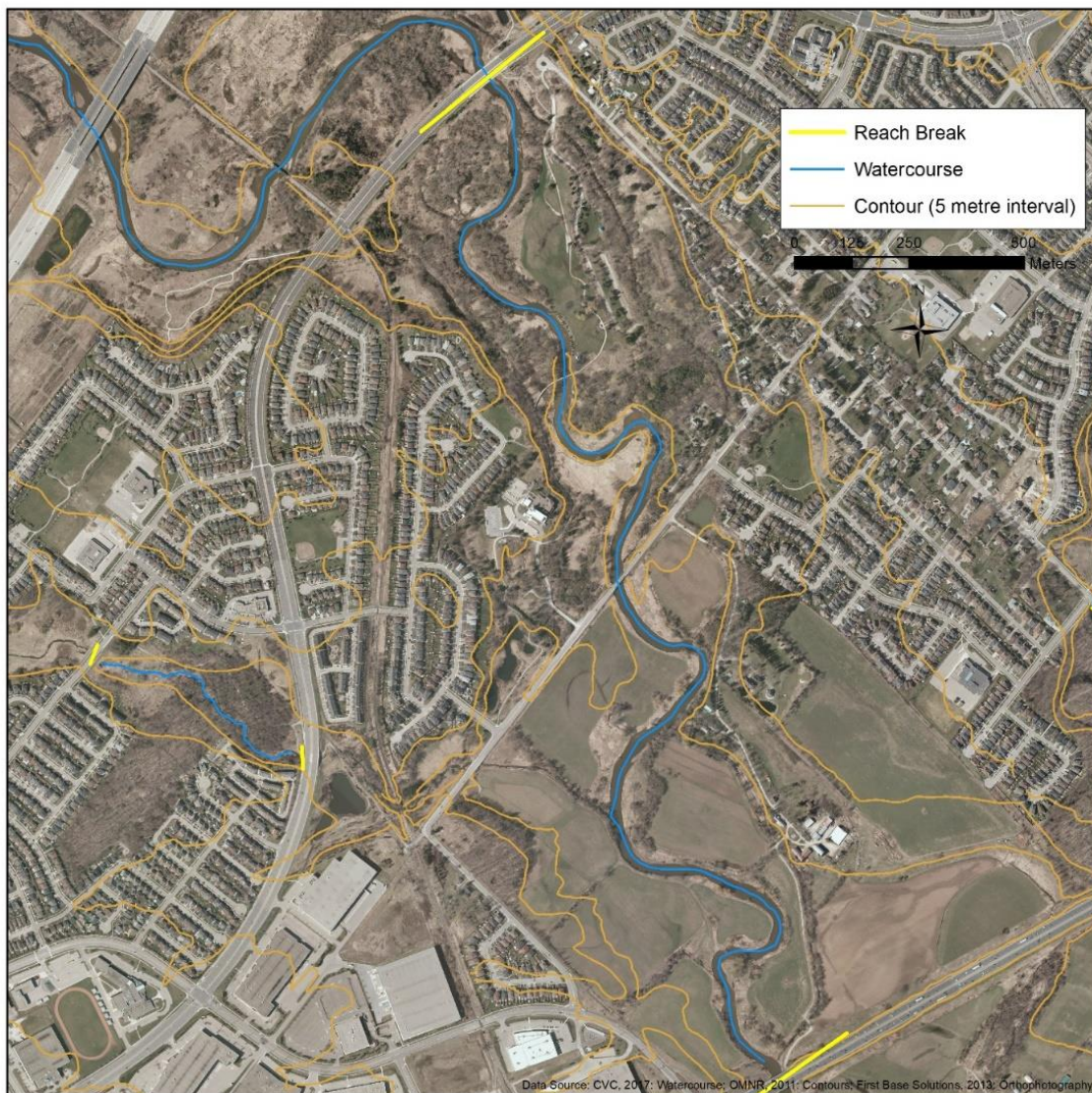
Figure 4.4 – Larger fluvial system with regular meandering tendencies (Reach CR11).
