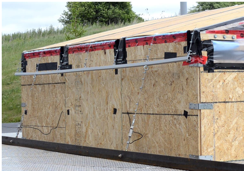
Figure 3.14 Windward face of the retrofitted reduced scale test specimen
