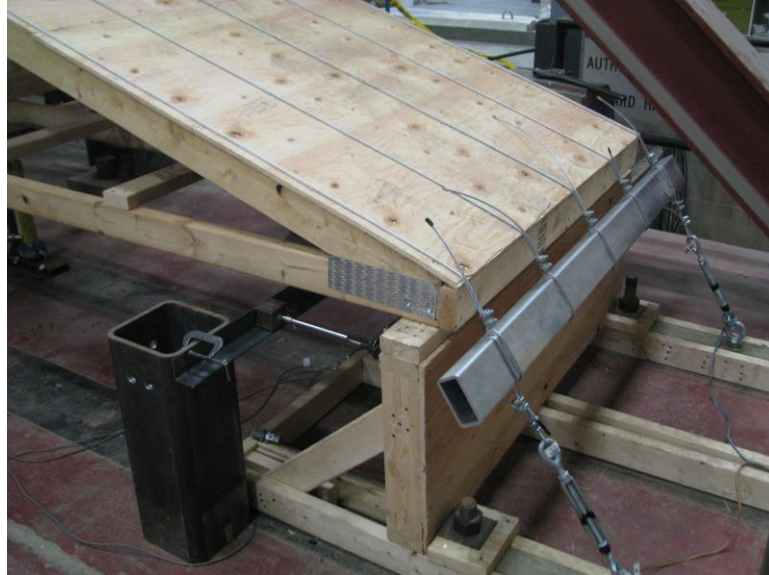
Figure 1.6 Sample roof strip and retrofit tested by Jacklin and El Damatty (2014)
