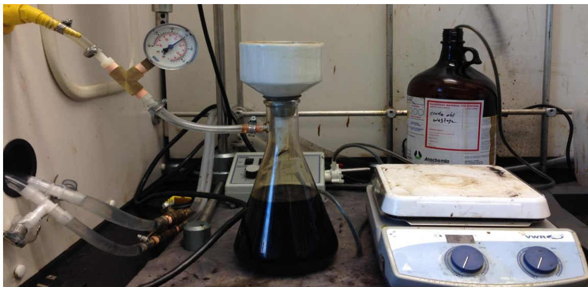
Figure 5-2 Schematic diagram of the experimental setup for asphaltene extraction.
