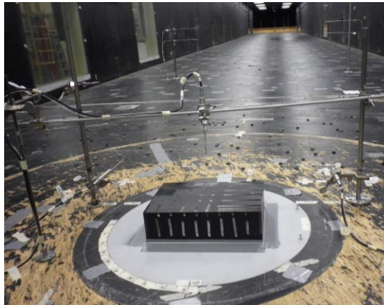
Figure 2-2: (a) Pressure tap locations for the 1/50 TTU building along with the Cartesian coordinate of the space and wind azimuth definition. (b) The planar image frames of PIV measurement near the TTU building model by Akon and Kopp (2016) (also indicated in plot (a)); (c) The point location m of the cobra probe velocity measurement (Wu and Kopp, 2016) (also indicated in plot (a)).
