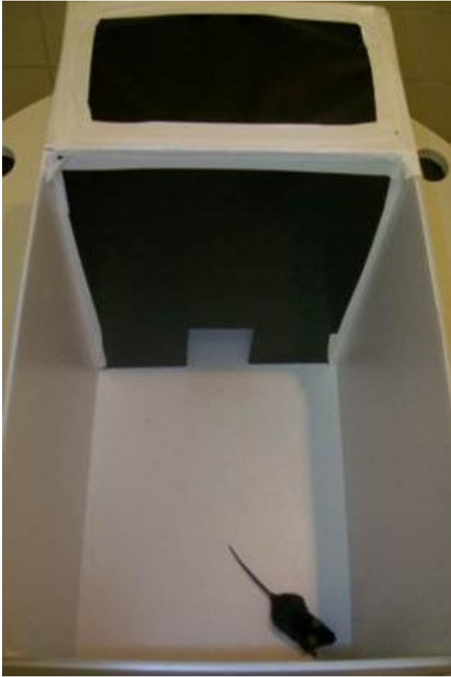
Figure 5: A photograph of the Light/Dark Box (LDB) used to assess stress- and anxiety-related endophenotypes in mice. A C57BL/6J mouse is shown in bottom right corner of the LDB. The LDB test measures the amount of time spent by a mouse in the light region (relative to the time spent in dark region). This measure is considered to quantify a mouse's explorative behaviour and can tell us something about the mouse's state of stress and anxiety.
