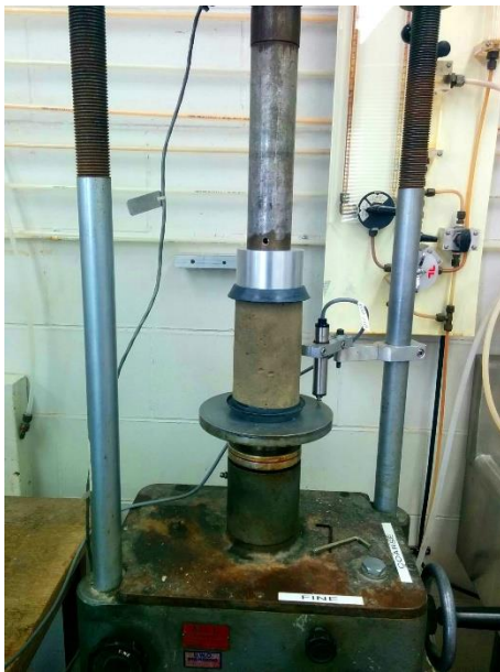
a. Unconfined compressive strength test
