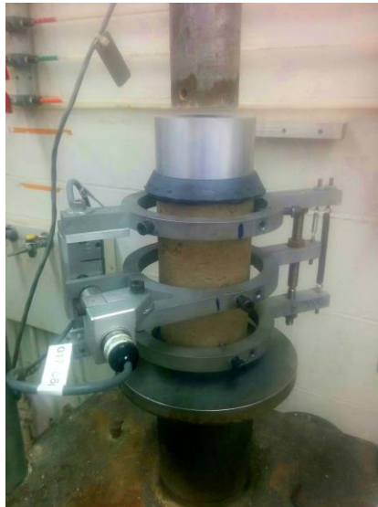
Figure 4.4 Determining static Poisson's ratio using a compressometer
