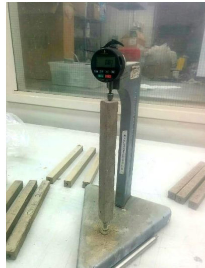
b. Length Comparator with sample
