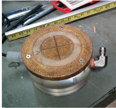
Figure 4.1 PRA device for measuring shear wave velocity
