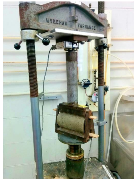
b. Split tensile strength test
