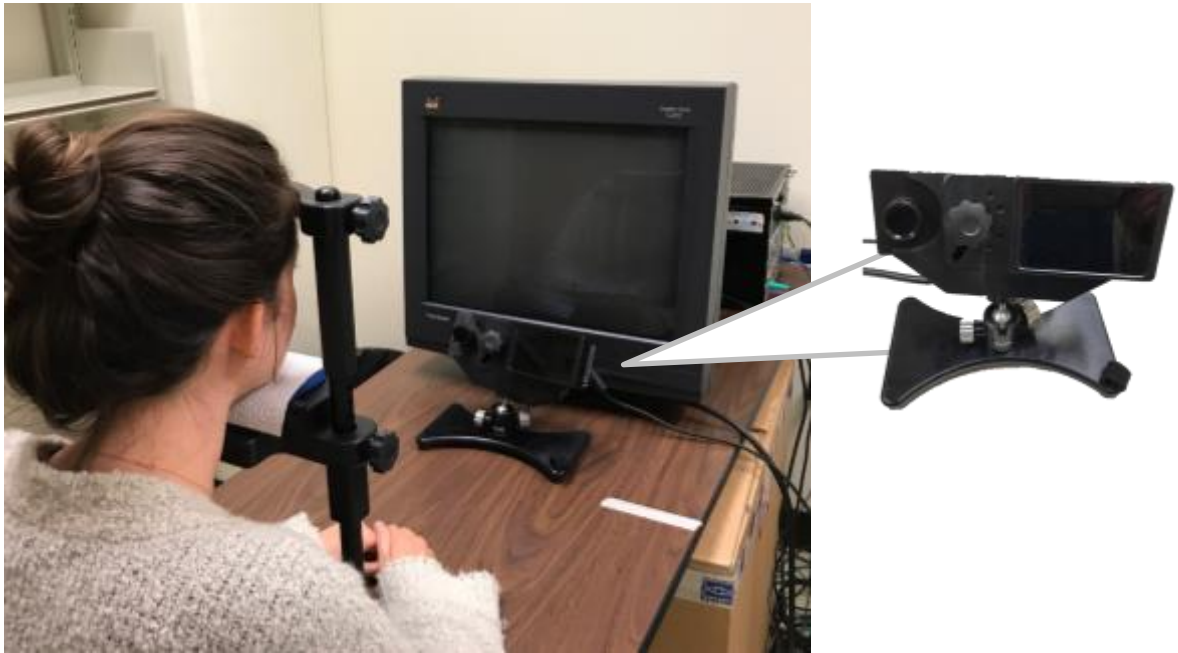
Figure 2.3. An image of the eye tracking set-up. Participants placed their head into a chin and forehead rest and looked forward at a computer screen while their spontaneous eye blink rate was quantified using the EyeLink 1000 core system via an infrared camera placed in front of them below the computer screen (shown in enlarged image).
