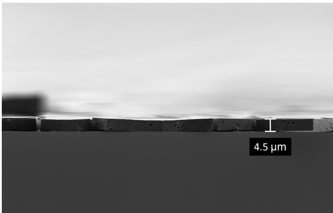
Figure S21. SEM of a cross-section of a thin film prepared by drop casting 6\mathbf{F}\text{-}[\text{Co}_2(\text{CO})_6]_2 onto a silicon wafer.
