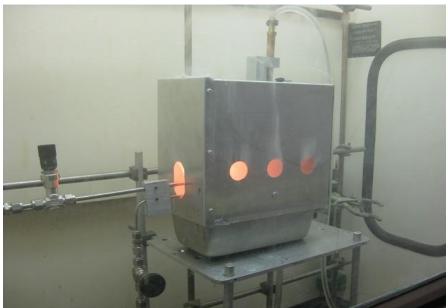
Figure S31. Photographs of the reaction setup (top) and burn box (bottom) used for the safe handling and disposal of \text{PH}_3 gas during this study.
