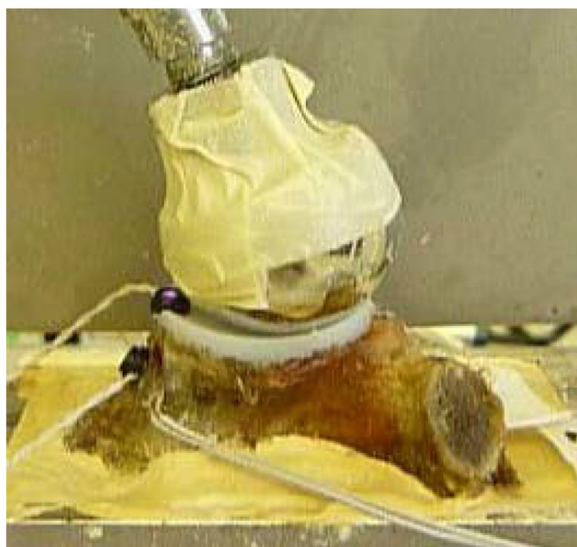
Fig. 2 The loading apparatus demonstrates a 30° loading vector with two optical trackers. One optical tracker is attached to the polyethylene and one is attached to the bone as a reference. The scapula is potted within the cement box. There is masking tape over the humeral ball to reduce potential reflection to the camera (not shown)
