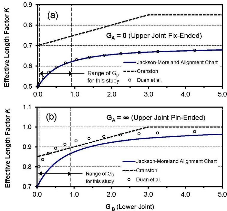
Figure 3: Comparison of effective length factors ( $K$ ) computed from different design equations when (a) the upper joint of the column is fix-ended; and (b) the upper joint of the column is pin-ended
