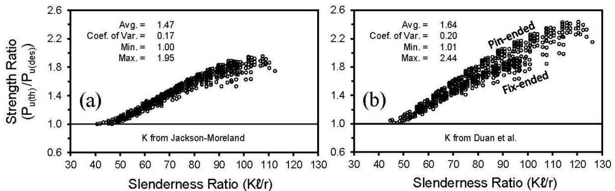
Figure 4: Effect of column slenderness ratio on strength ratios for load cases 1, 2, 3 and 4 ( $n = 648$ ) calculated using (a)  $K$  from Jackson-Moreland Alignment Chart; and (b)  $K$  from Duan et al.
