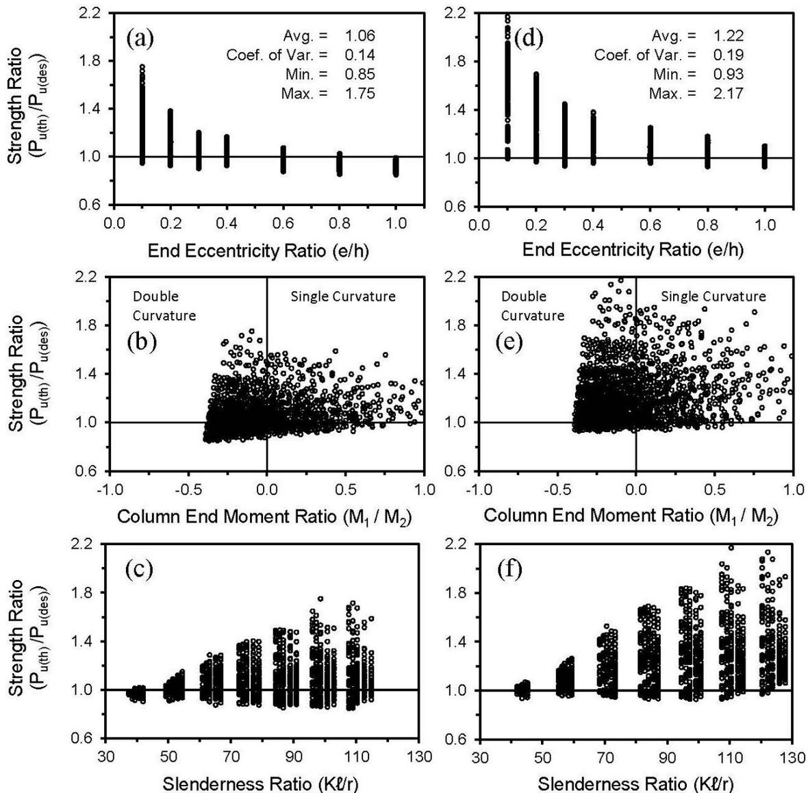
Figure 5: Effects of variables on strength ratios for load cases 5 and 6 ( $n = 1520$ ) calculated using K from Jackson-Moreland Alignment Chart: (a) end eccentricity ratio ( $e/h$ ), (b) column end moment ratio ( $M_1/M_2$ ), (c) slenderness ratio ( $Kl/r$ ); and K from Duan et al. equation: (d) end eccentricity ratio ( $e/h$ ), (e) column end moment ratio ( $M_1/M_2$ ), (f) slenderness ratio ( $Kl/r$ )
