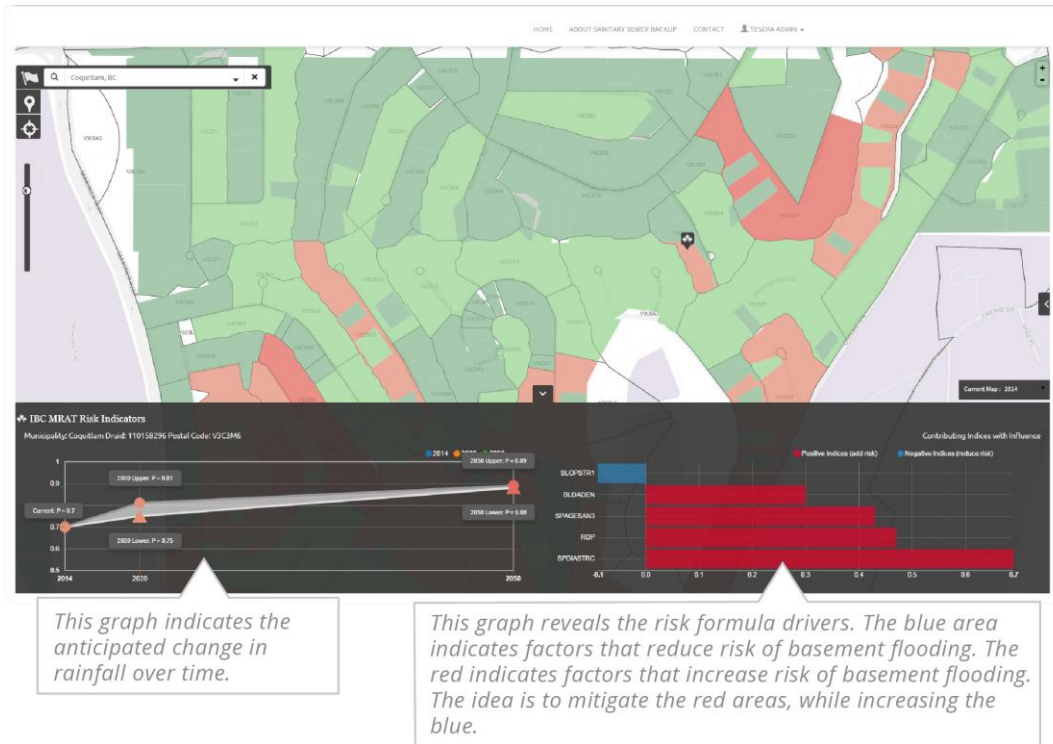
Figure 3: Sample View of FLOOD Risk Map of Coquitlam, With Information Graphs at Bottom
