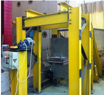
Figure 1: Impact apparatus (Bayoumy 2014)
