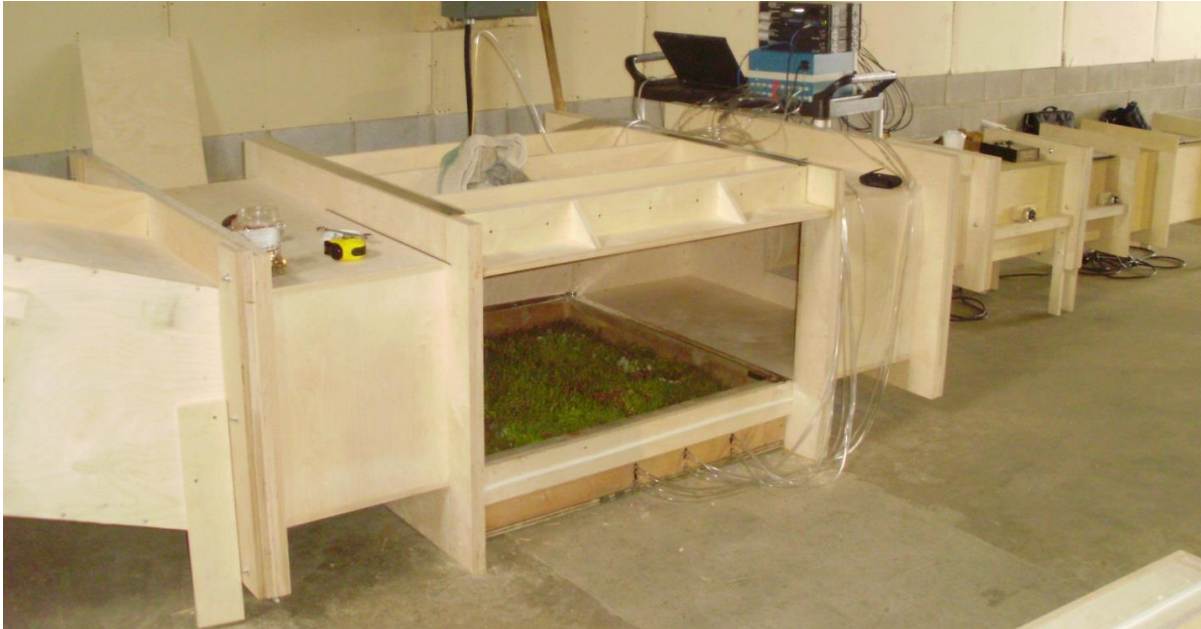
Figure 2: Green roof sample within the pressure chamber (note the door has been removed for this photo)
