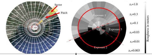
4-Obtain wind profiles at the site for wind blowing from various angles and find the best matching wind tunnel profile. Reproduce all the geometry of all the surrounding buildings within a half kilometer of the study building
