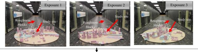
5-Measure wind loads from the aerodynamic or aeroelastic wind tunnel tests
