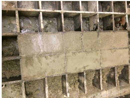
Figure 2: Mortar Specimens with different DE concentrations cast
