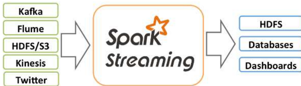
Figure Spark Streaming architecture
