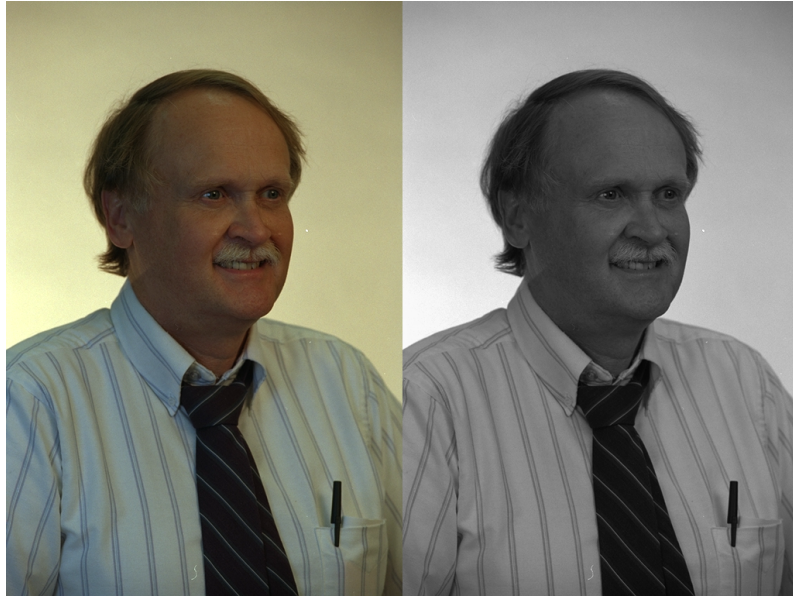
Figure 22: OpenCV RGB Image to Grayscale. Left image is the original image. Right image is the gray scale image. [26][27]
