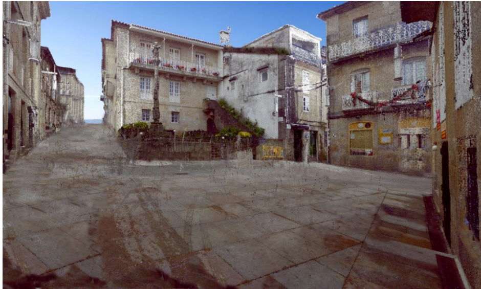
Fig. 57. Raw LiDAR scan rendered in 'ToView'. Real time open GL screen capture, with post processing. 'Calle Baron' in Pontevedra, Spain.
