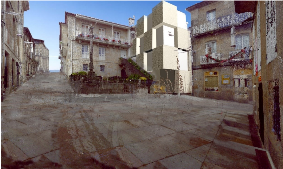
Fig. 60. LIDAR scan rendered in 'ToView', merged with the artificially generated. Post-processed PBR Real time open GL screen capture.
