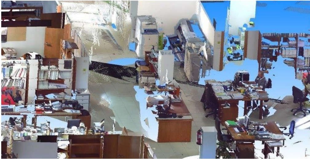
Fig. 06. View of the unfiltered point cloud data.
