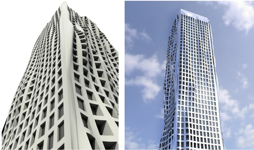
Fig. 83. Tower design resembling the Beekman Tower, this time generated by the GA algorithm, and rendered in VRay.
