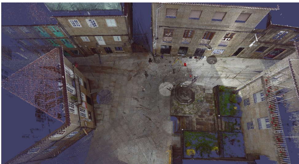
Fig. 55. PBR 3D visualization of a real urban environment, previously scanned using LIDAR technology.
