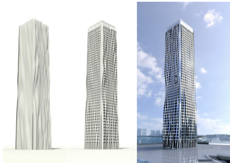
Fig. 82. Design process of making windows and rendering over the selected auto-generated surface.
