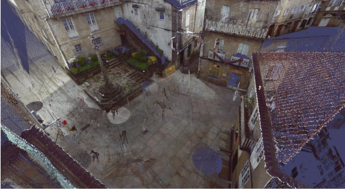
Fig. 08. ToView visualization from a LIDAR scan using 'Faro Focus 3D', of a small historical urban environment.
