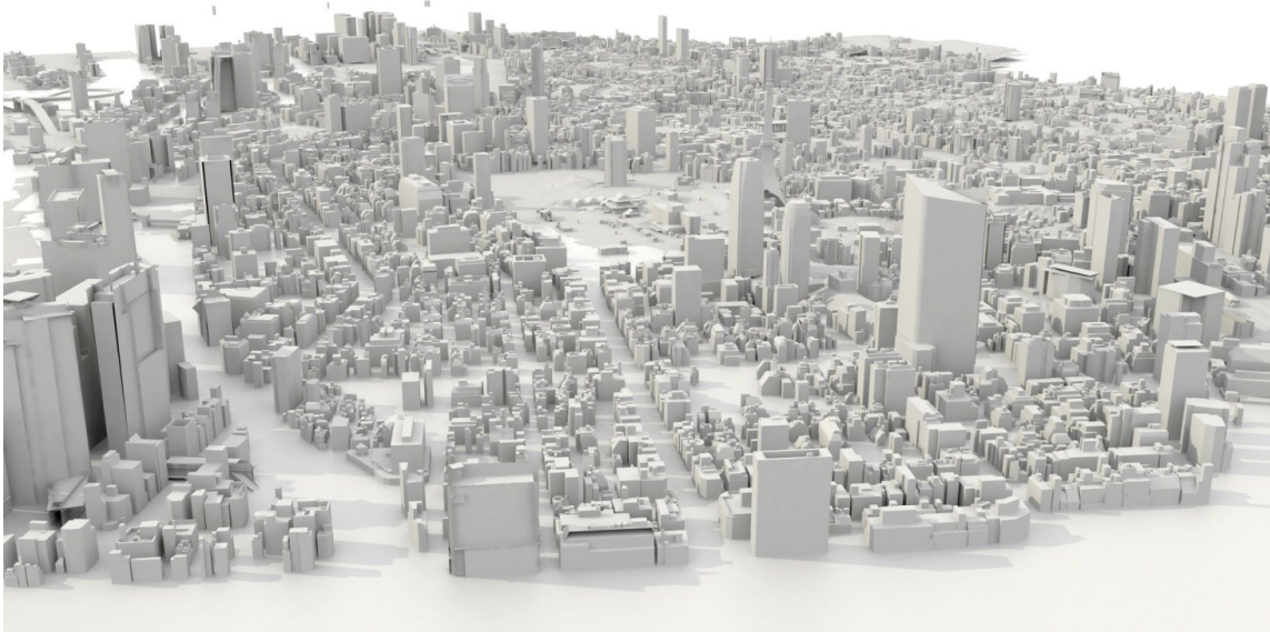
Fig. 91. Polygon mesh of photogrammetric 3D Model of Minato Ward skyline.
