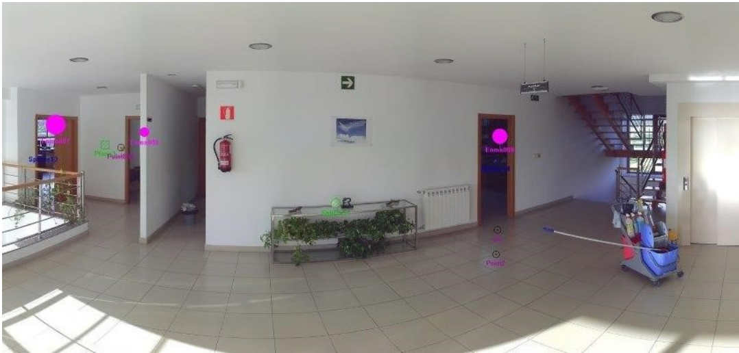
Fig. 05. Software view with spheres, common points and planes.
