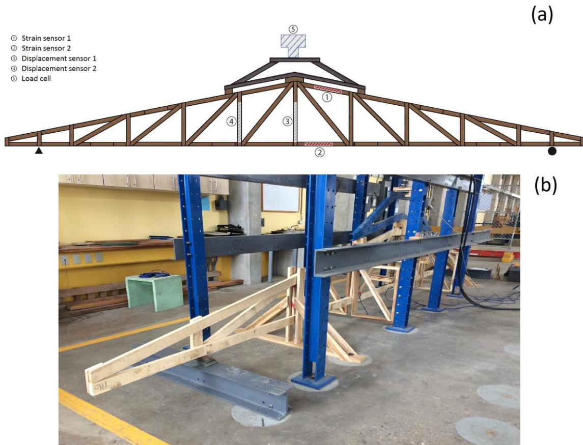
Fig. 2. System for application of loads in truss tests (a). Restrictive elements used to avoid sideways motion of trusses during tests (b).
