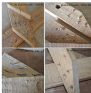
Fig.3: Types of fastener failure of nail and screws in H. alchorneoides joints at 30° (a and b, respectively) and G. arborea joints at 30° (c and d, respectively).
