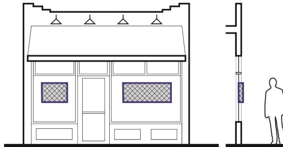
Display window sign diagram illustrating proper proportion and placement on the building.
