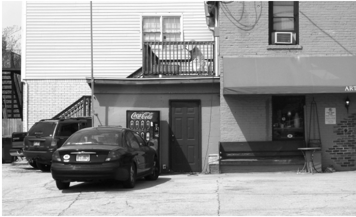
Figure F1 - This addition is in a good location, as it is behind the main block of the building and slightly recessed, so as not to obstruct or detract from the view of the historic building.
