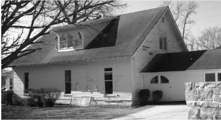
Figure F15 - This is a recommended rear addition because the massing and scale are both smaller than that of the historic house, making them less visible when looking at the front of the historic house. The graphic below gives examples of appropriate and inappropriate location and scale.
