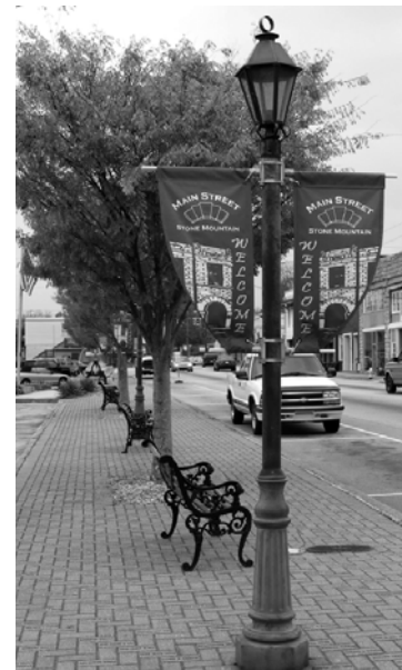
Figure J5 - The street lighting installed in the commercial area has historic design elements, but does not attempt to look historic. The lighting is also not too large in scale when compared to the buildings and other street furnishings around it.
