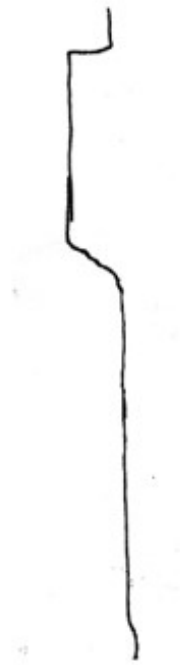
Molding of the door frames of the doors in the main house.
