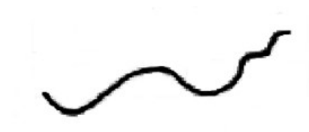
Molding surrounding the panels on the bottom of the French casement windows of room 101, 103, 104, and 202.
