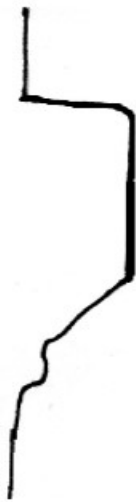
Pilasters of the fireplaces in rooms 103, 104, and 201-204.
