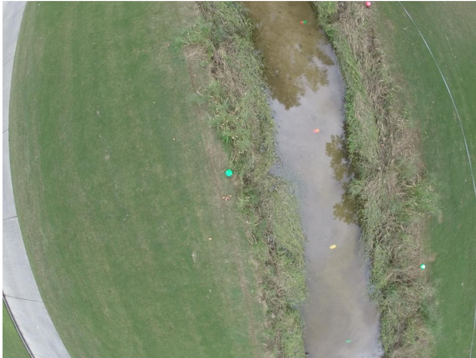
Figure 2.1: Image taken during flight at the DHGC site location showing the GCPs placed along the reach banks and in the stream bed
