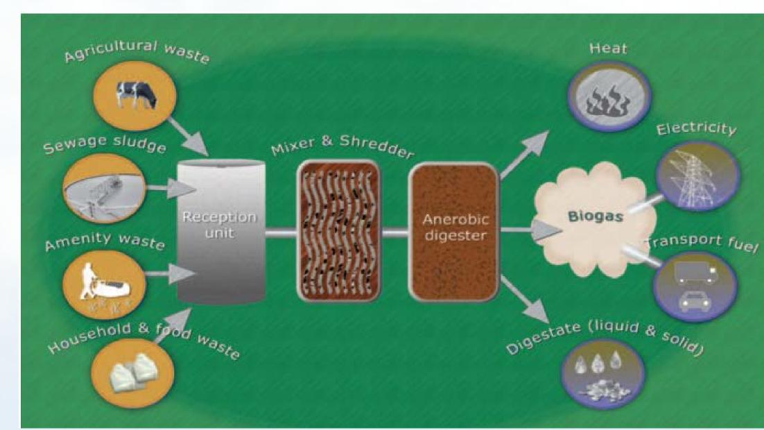
Figure 3. Intake, processing, and output of a biogas plant<sup>[2]</sup>
