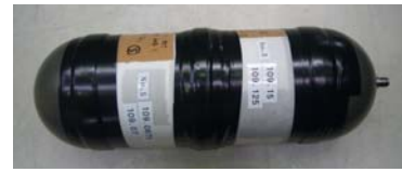
Fig. 4(a) Photo of a small-sized pressure-tight housing for hydraulic pressure tests with two jointed ceramic cylinders
