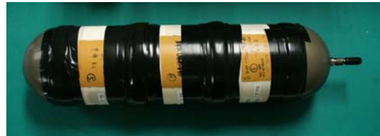
Fig. 4(b) Photo of a small-sized pressure-tight housing for hydraulic pressure tests with three jointed ceramic cylinders
