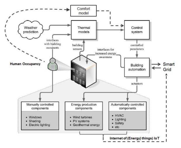
Fig. 2 Smart bulding component and connection to a smart grid. (Adapted from [9] & [10])
