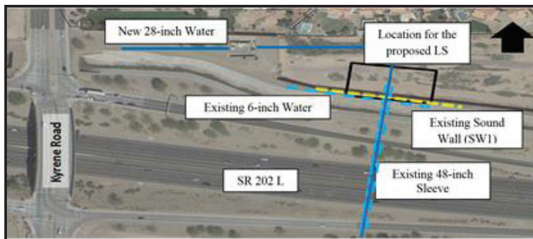
Fig. 2. Schematic drawing of 28-inch Force main project
