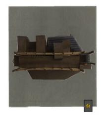
The northwest skin of the building is more permeable due to the benefits of cooler air and less sun exposure. Most of the interior spaces are situated along this shaded side of the building, which also provides scenic views of the Florida Bay.
