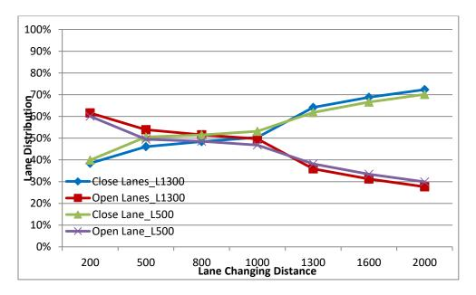
Figure 4-18 Lane Distribution Ahead of Work Zone
