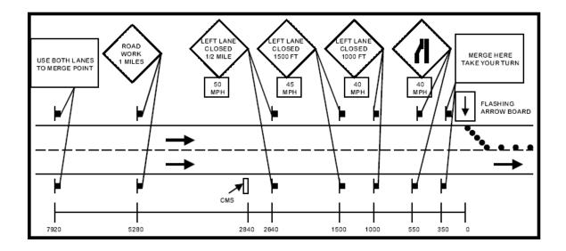
Figure 2-2 Late Merge Traffic Control Plan
