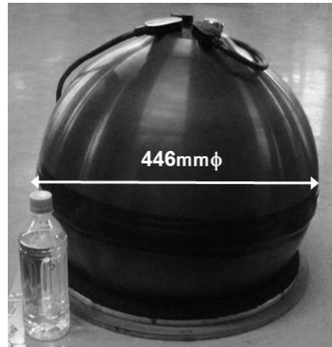
Fig. 4. Photograph of the ceramic pressure-tight housing designed for OBS. It can withstand hydraulic pressure of 110 MPa.
