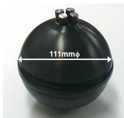
Fig. 3. Photograph of a small model of a ceramic pressure-tight housing for OBS.
