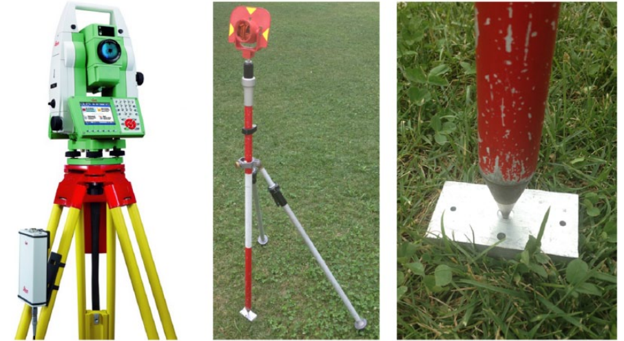
Figure 2. Instruments used for data acquisition: total station, prism, pole and base
