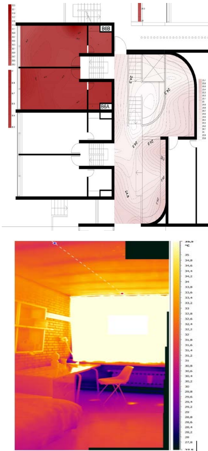
Fig. 9. Distribution of temperature (left) in B6b room (top) and B6a (bottom) compared with the common space (in the middle) of the “Aquilone” building– 14/07/2016. Thermal image of B6b room - 14/07/2016 (right).
