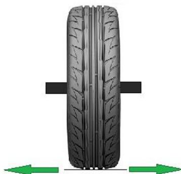
Figura 4.8 – Lateral Runout. (15)
