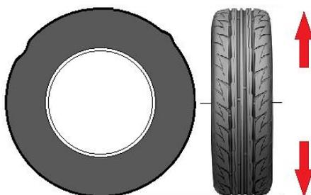
Figura 4.7 – Radial Runout. (20)
