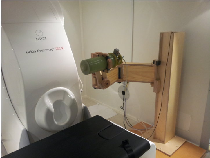
Figure 4.4: Elekta Neuromag ® TRIUX together with the single channel high- T_c SQUID-based MEG system mounted on a wooden stand.
