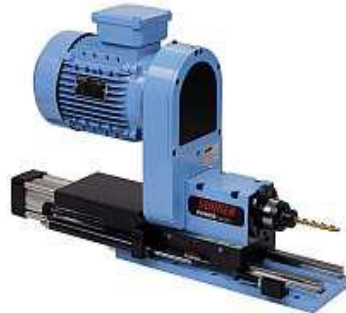
c) An example of POWER machining unit mounted on a sliding unit (BEX 15/UA 15)
