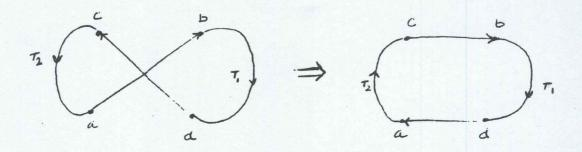
Figure 1: We tweak a pair of edges by replacing them by two edges, one that joins the heads and one that joins the tails. Half the tour is then reversed to yield a new directed tour. A tweak is advantageous if by performing the tweak we reduce the length of the tour.
