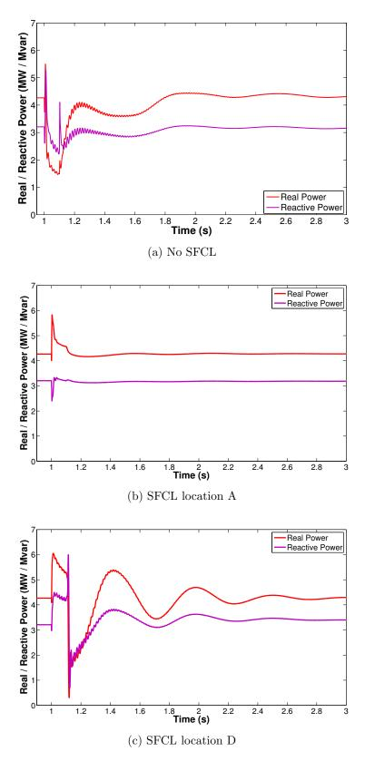
Figure 4.7: Instantaneous real and reactive power delivered by 4 MW generator in the right subsystem for fault F3, with SFCL resistance of 1  $\Omega$
