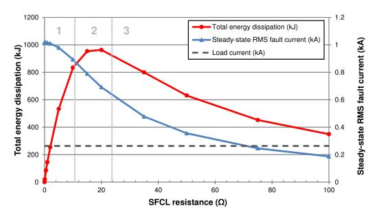
Figure 5.2: Energy dissipation and fault current limitation for various SFCL resistance values (at 33 kV side of DG transformer)
