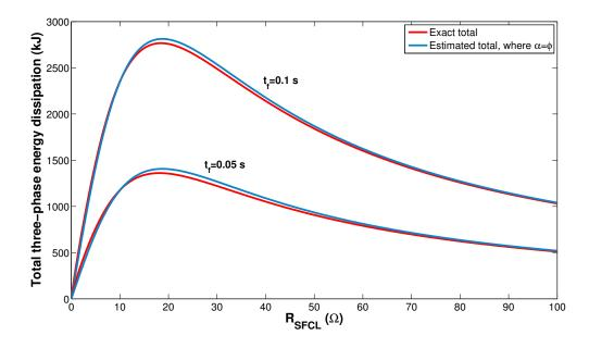
Figure 5.5: Total three-phase energy dissipation: exact vs. approximation
