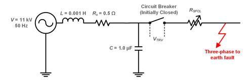
Figure B.4: SFCL located downstream of circuit breaker
