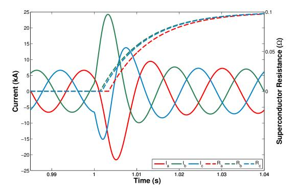
Figure A.1: Typical per phase SFCL resistance characteristic and effect on fault current
