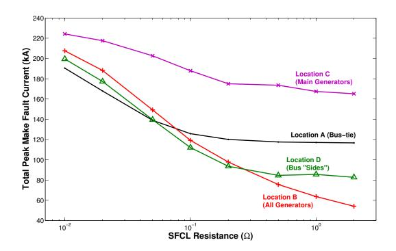
Figure 4.4: Total peak fault current for fault F1
