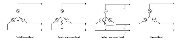
Figure 2.3: Comparison of system earthing types, shown at generator or transformer star-point connection
