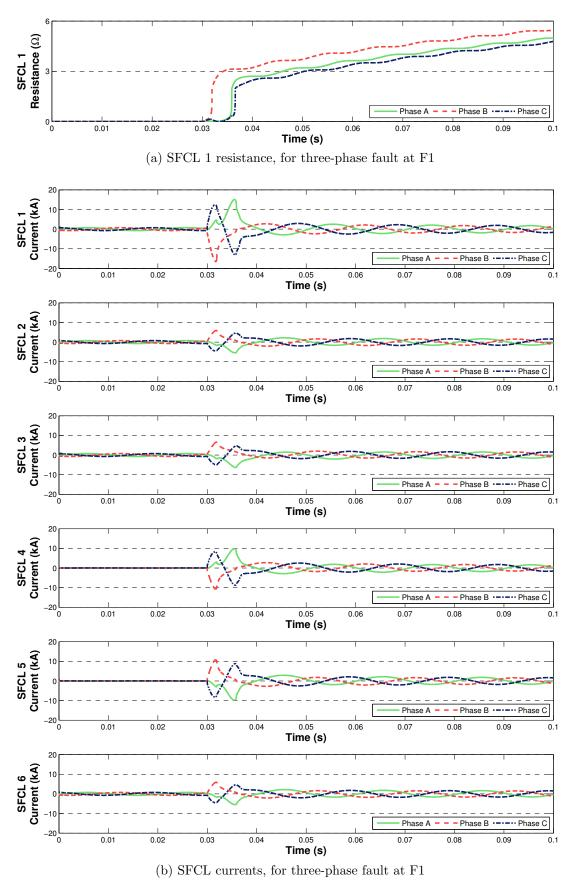
Figure 7.6: SFCL resistances and currents for three-phase fault at F1
