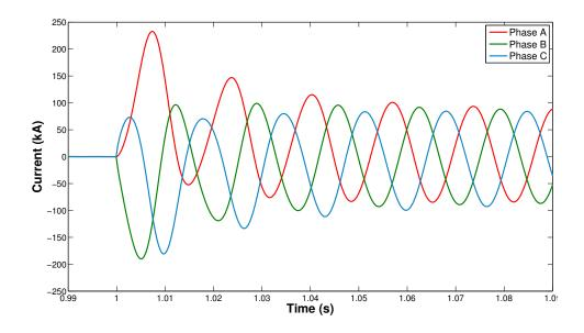
Figure 2.10: Short-circuit fault on the 690 V bus
