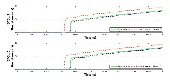
Figure 7.7: SFCL 4 and 5 resistances, for three-phase fault at F2
