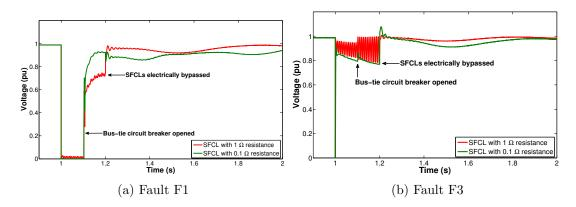
Figure 4.8: 690 V bus voltage for SFCL location D, for faults F1 and F3
