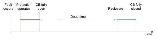
Figure 2.2: Typical autoreclose timing for a transient fault
