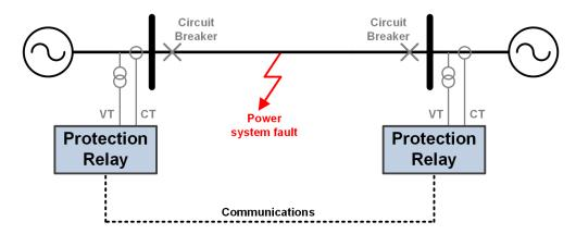
Figure 2.5: Typical two-terminal differential protection arrangement
