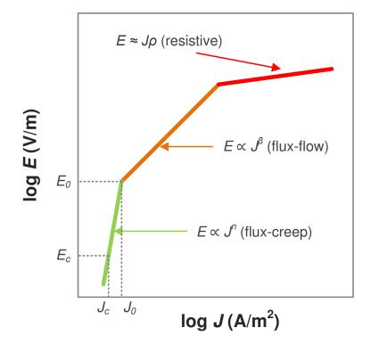
Figure 6.1: Superconductor E-J characteristic (from [PCL<sup>+</sup>00])
