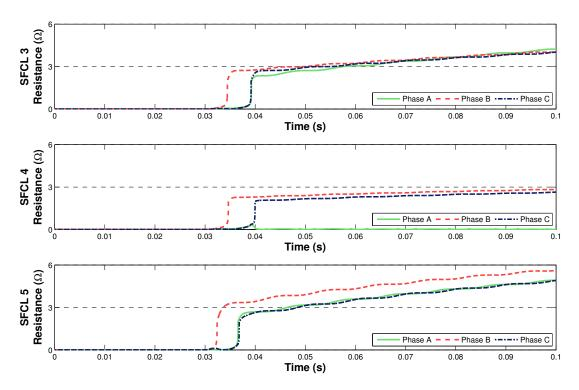
Figure 7.10: SFCL 3-5 resistances, for three-phase fault at F2, without the incoming feeder at SFCL 1
