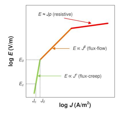
Figure A.3: Superconductor E-J characteristic (from [PCL<sup>+</sup>00])
