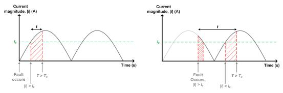
(a) Sufficient energy dissipation for quenching (b) Quenching in first cycle "missed" due to low energy dissipation
