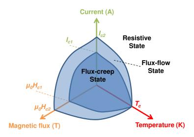
Figure 3.4: Conditions needed for superconductivity [PC98, BHH<sup>+</sup>11]
