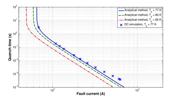
Figure 6.4: SFCL model current-time characteristics (analysis and simulation). Fault current for DC simulation is the initial fault current from a constant DC voltage source.
