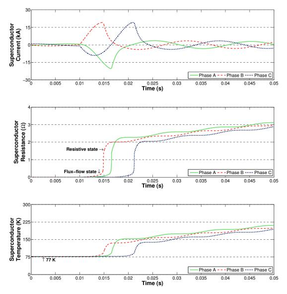
Figure 3.6: Resistive SFCL operation
