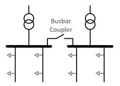
Figure 3.1: Opening a busbar coupler
