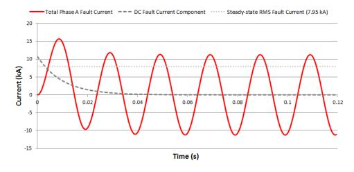
Figure 2.4: Typical fault current waveform (only phase A shown for simplicity)
