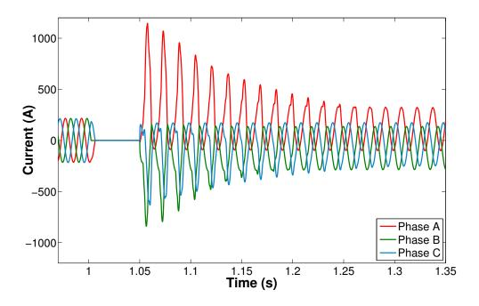
Figure 4.11: Transformer inrush current for 350 kVA marine transformer
