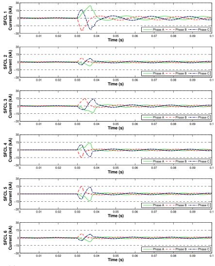
(b) SFCL currents, for three-phase fault at F1, during backup operationFigure 7.8: SFCL backup operation for three-phase fault at F1
