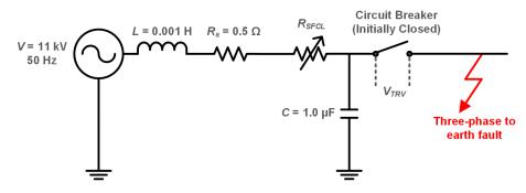
Figure B.1: Circuit used to examine effect of SFCL on TRV
