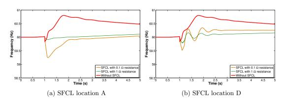
Figure 4.10: System frequency for Fault F3
