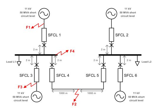
Figure 7.3: Example 11 kV AC distribution system
