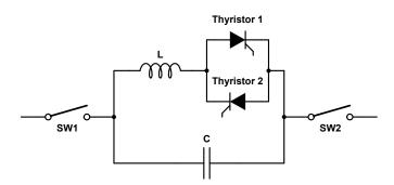
Figure 3.2: Typical resonant fault current limiter [Kar92]
