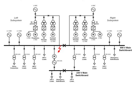
Figure 2.9: Typical marine AC electrical system
