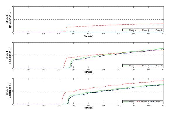
Figure 7.11: Incorrect quench of SFCL 3 for Fault 2, during reduced fault level
