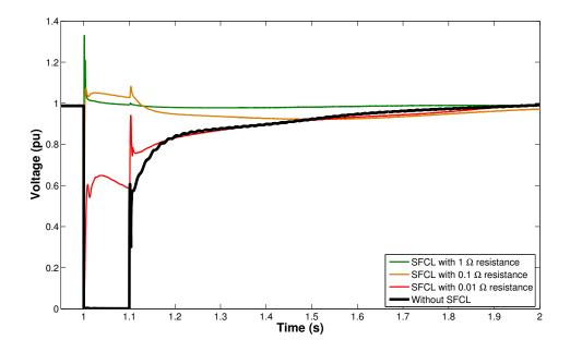
Figure 4.6: 690 V bus voltage for SFCL location A, for fault F1 (or F3)
