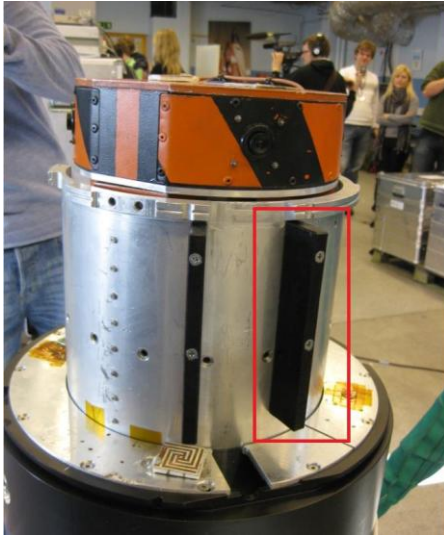
Figure 8: Only Suaineadh part found during recovery mission: bracket from magic hat.
