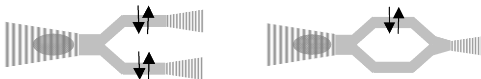
Figure 5: Schematics of other possible simple devices. (Left) Separation of information on to two frequency separated channels — depending on direction of field applied to individual arms their output frequency can be up-shifted, down shifted or unchanged with respect to the input. (Right) A device such as might be used to explore plasmon interferometers.
