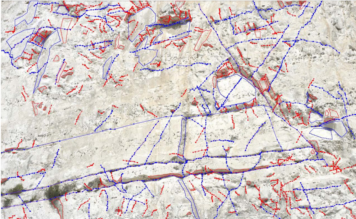
Figure 4-9. Orthoimage (striking 085°) showing large scale structures (>1 m, blue) and small scale structures (<1 m, red).
