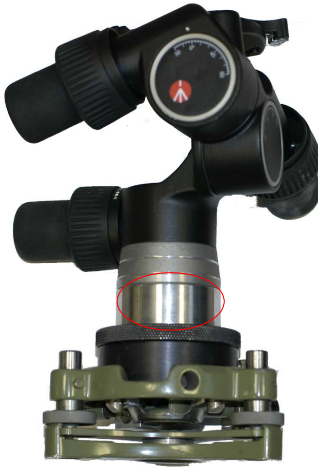
Figure 4-62. Geared camera head fitted with tribrach attachment (highlighted in red). The screw fitting for the geared head was modified so that it may be interchanged between normal photographic tripods and surveying tribrachs.
