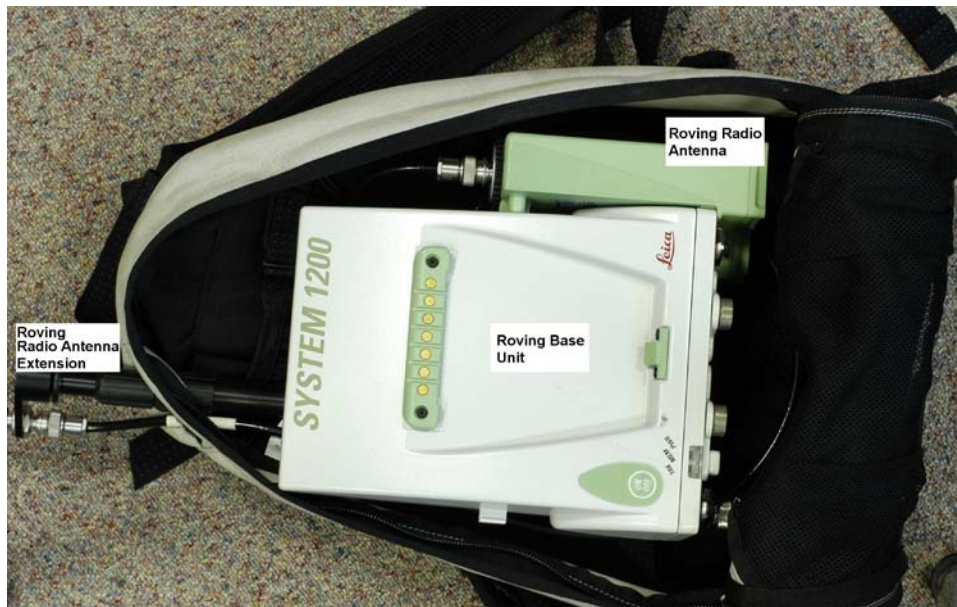
Figure 3-9. Roving GPS unit in backpack.
