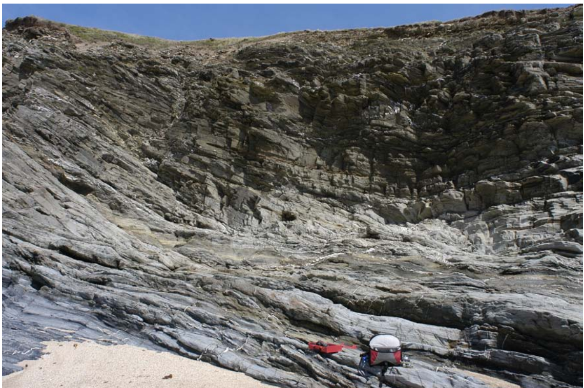
Figure 4-23. Photograph of cliff face at Blue Rocks, Gunwalloe, UK, looking north (cliff height from beach is 12 m). Folding is evident in the centre of the photograph, and wedge failures can be seen in the upper sections of the face.
