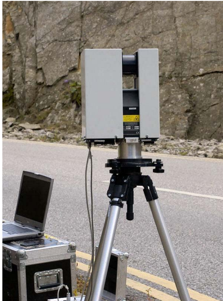
Figure 3-12. Photograph showing the Leica HDS4500 phase shift laser scanner. A mirror in the centre of the scanner spins reflecting the laser emitted vertically from the base of the scanner.
