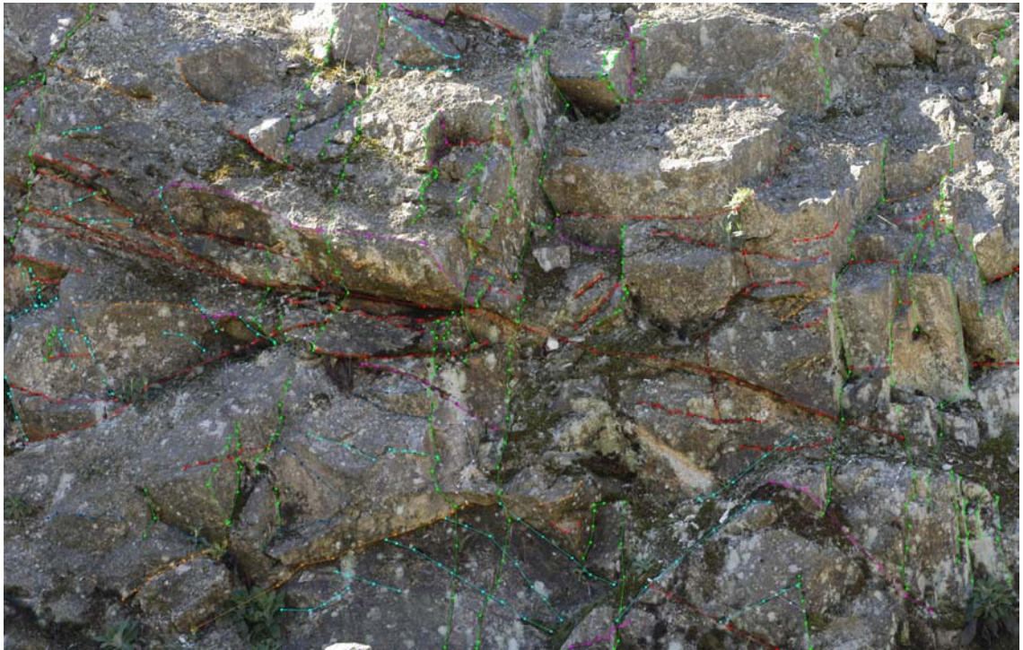
Figure 5-15. Photogrammetric discontinuity trace length identification, Tremough Road cutting, Penryn, Cornwall, UK (~3 m wide, 2.5 m high rock face, looking south).
