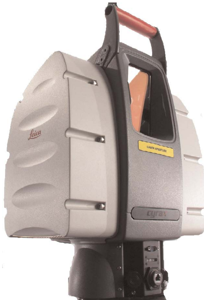
Figure 3-11. Leica HDS3000 (from Leica, 2005). The laser is emitted through main window (pictured). A second window at the back of the scanner is used for capturing points at an angle of less than 40° from vertical.
