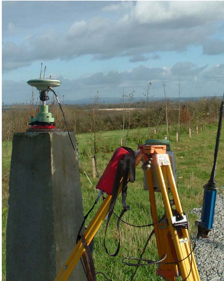
Figure 3-7. Differential GPS Equipment – base station. The base station is setup over a known position that has previously been surveyed and begins to receive satellite signals. The location of the base station is input into the machine so it can then compare it with the positions that it calculates for itself using the satellite code, hence calculating the positional error for each moment in time. This error is then transmitted to the roving GPS unit so that it can calculate its position accurately.
