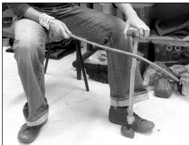
Fig. 24: The bow drill being used on one of the copper axe blanks (source: Author)
