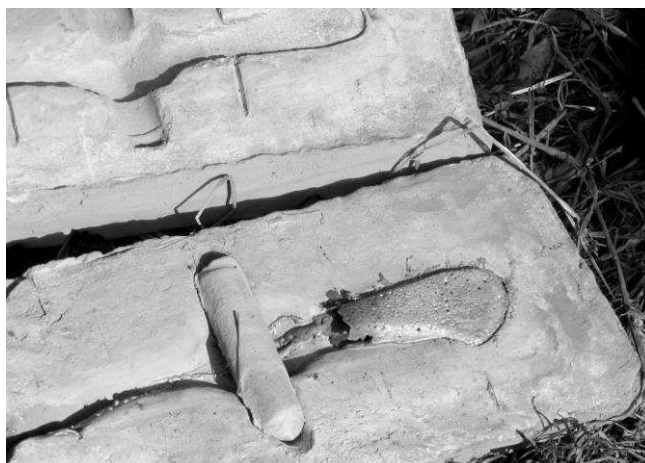
Fig. 17: The partly filled mould after casting session 1 (source: Author)
