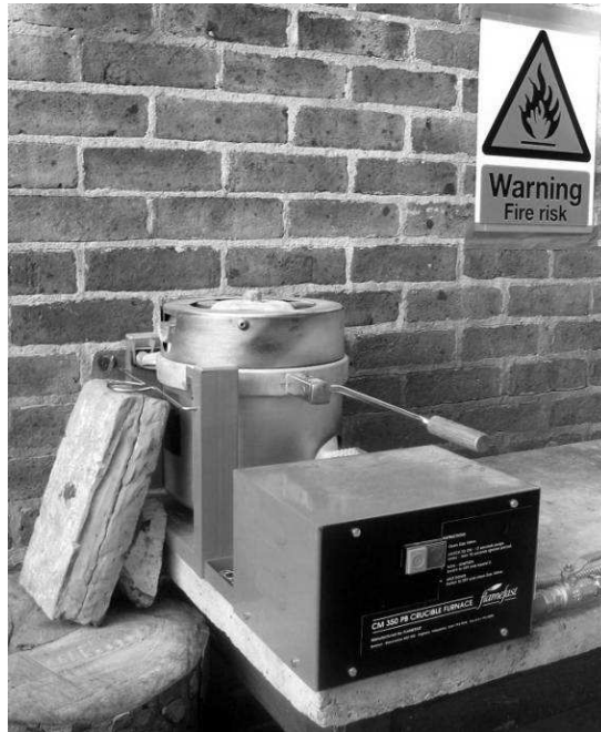
Fig. 22: The gas fired furnace (source: Author)
