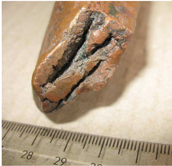
Fig. 93: The axe cutting edge split open, which indicates that it was forged together (photo: Author)
