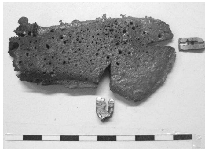
Fig. 32: The object cast in session I with the two samples taken for metallographic analysis from the cutting edge (sample 1) and the side (sample 2) (source: Author)
