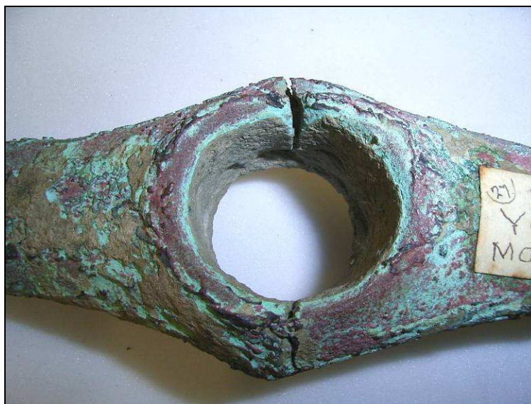
Fig. 84: Two early cracks on either side of a shaft-hole of an axe-adze (source: Author)
