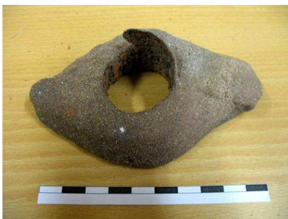
Fig. 27: Experimentally cast axe from the clay core series (source: Author)
