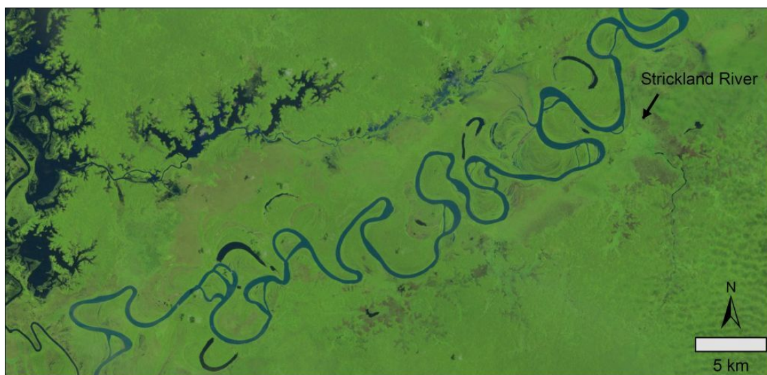
Figure 5.1: A sand-bed reach of the Strickland River in Papua New Guinea. Rapid bend extension here leads to wide scroll-slough spacing and associated initiation of chute channels, resulting in a planform dynamic and pattern that is transitional between single-thread meandering and braided (see Chapter 2).
