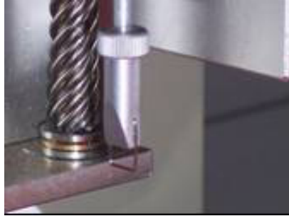
Figure I.2: The profile probe head for the Kawabata surface tester
