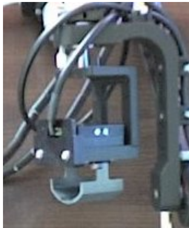
Figure 6.7: The force transducer (centre) attached to the curved force plate (below), and the gimbal (above, right) which links to the force-feedback device.
