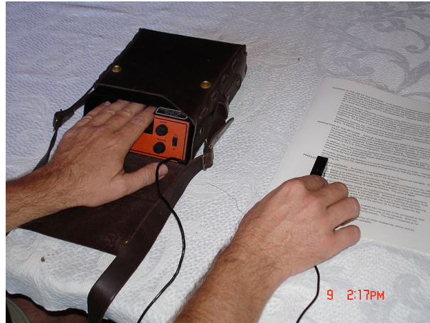
Figure 2.11: The Optacon in use ( Image source: Wikimedia Commons )
